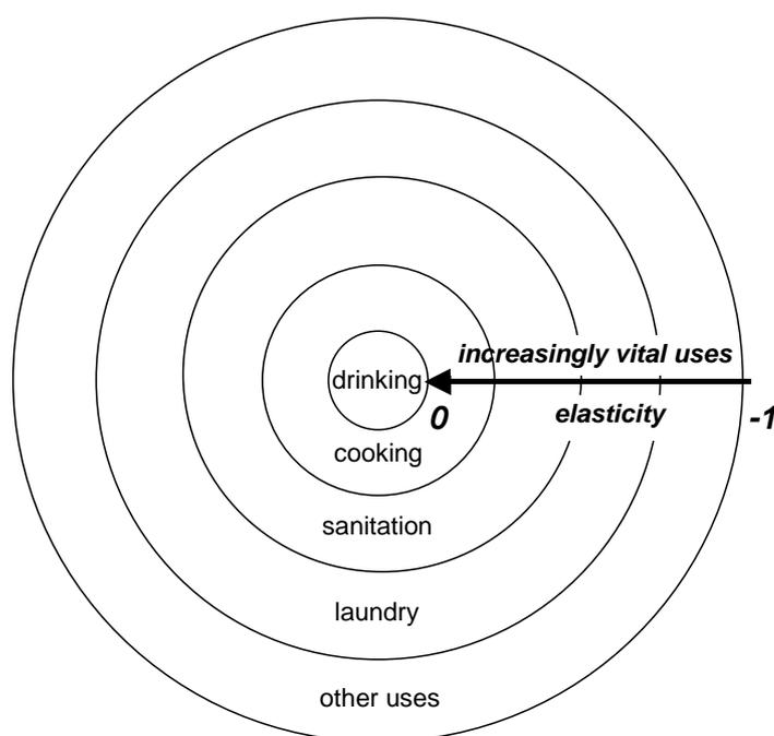
Figure 4.1: Schematic figure of different uses of domestic water and their elasticities of demand (Savenije & Van der Zaag, 2002)
